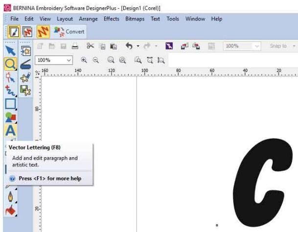
4. Select the letter then left click on the fill icon, the 'paint pot' on the left-hand tool bar. This opens a fly out toolbar offering different fill types. Select 'pattern fill'.
