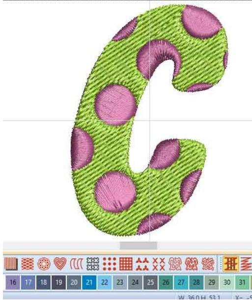
11. Select the embroidered letter and go to 'Object Properties' to change fill types and change colours to the thread colours that you wish to use. Each spot for example in this design could be a different colour!
